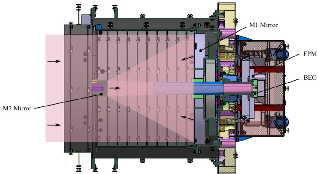
Figure 2: Optical layout of the CHEOPS telescope
