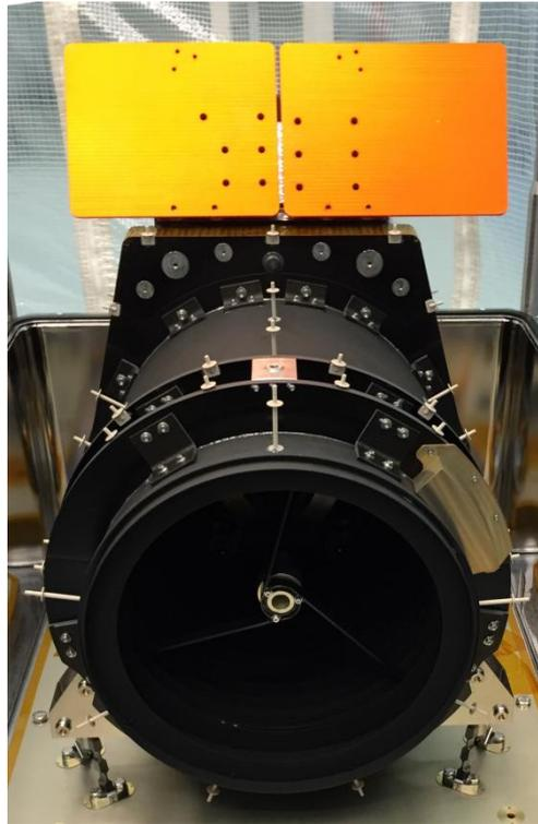
Figure 4: Structural and Thermal CHEOPS OTA model
