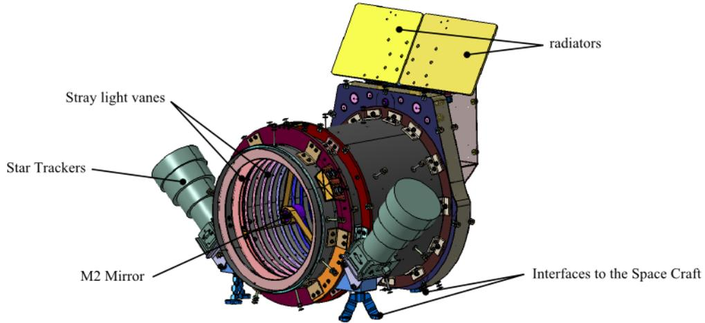
Figure 1: Overview of the CHEOPS OTA supporting the M1 and M2 mirrors, the Back End Optics (BEO) and Focal Plane Module (FPM).
