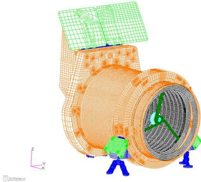
Figure 3: Overview of the Finite Element Model of the CHEOPS OTA
